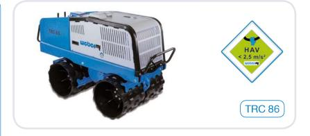
For compaction of the most difficult soil, trench rollers like the TRC are recommended. They are mainly used for the compaction of cohesive soil, in trenches and around pipelines, when compacting foundations and backfill and in road construction. Especially on difficult, cohesive and moist soil they have many advantages.
